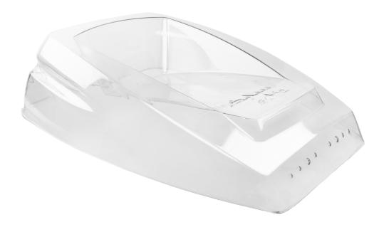
Thermoforming LEXAN™ EXTRITE™ sheet, a polycarbonate material, is a manufacturing process where a plastic sheet is heated to its softening temperature, formed to a specific shape in or over a mold by using vacuum, and trimmed to create a usable product.
